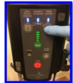
STEP 5: Press 'Prime System' on HICP200
