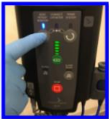
STEP 3: After zeroing the pressure transducer in the patient monitor, Press Zero Patient Monitor on HICP200
