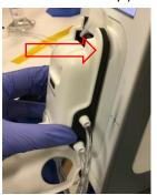
c. Using your thumb, push the cassette flat against the front cover of the Control Unit. See below.
