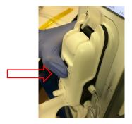
d. While holding the cassette flat against the front cover lever, press the cassette downward into the operating position.
