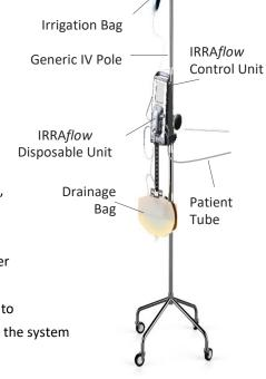
Settings can be changed on the user interface of the Control Unit. The pressure sensors can be calibrated at any time by using the calibration knob on the Tube Set cassette.
