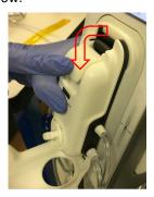
11. Press the cassette lever firmly downwards to lock the cassette into position. Raise the cassette lid to magnetically latch to the face of the Control Unit.
