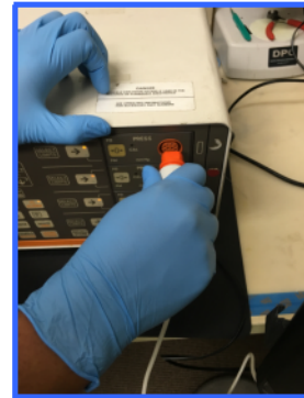
Remove Monitor Cable from patient monitor
