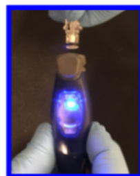
STEP 4: Connect ICP Catheter Connector to Patient Cable Module
