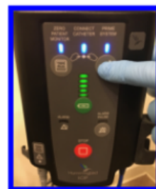
STEP 5: Press 'Prime System' on HICP200
