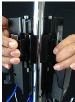
Fig. 5 Clamp attached to equipment pole
